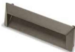
Maniglia 581 ad incasso - finitura bronzo-titanio anta da L 15 a L 30 → passo 67 mm anta da L 30 a L 90 → passo 126 mm Recessed handle 581 - bronze-titanium finish door from W 15 to W 30 → span 67 mm door from W 30 to W 90 → span 126 mm
