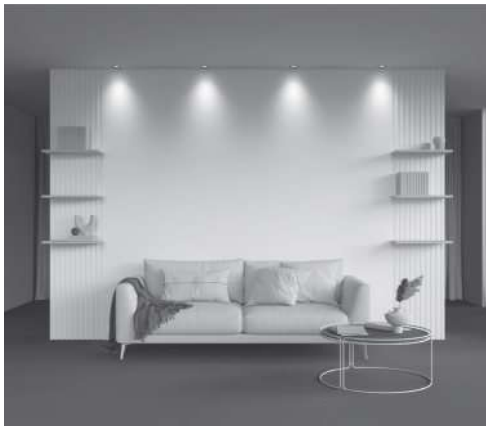
Recessed light source for anti-glare effect.
